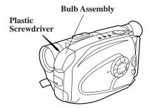
2. Pull on the sides of the bulb assembly and remove it from the camcorder *as shown*.
